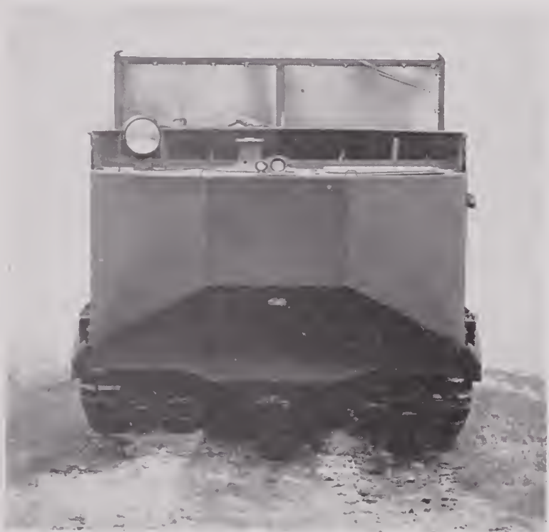
FIGURE 55. Front view of M-29C Weasel, showing final design of bow cell.
